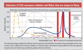
characteristics of infrared rays emitted by objects other than flames.
